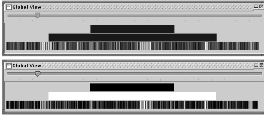
Figure 3. The top view shows clustering loss and the bottom view displays excess coverage loss for an R*-tree indexing 8-D clustered point data. These views have been extracted from the user interface and placed side by side to highlight the correlation.
