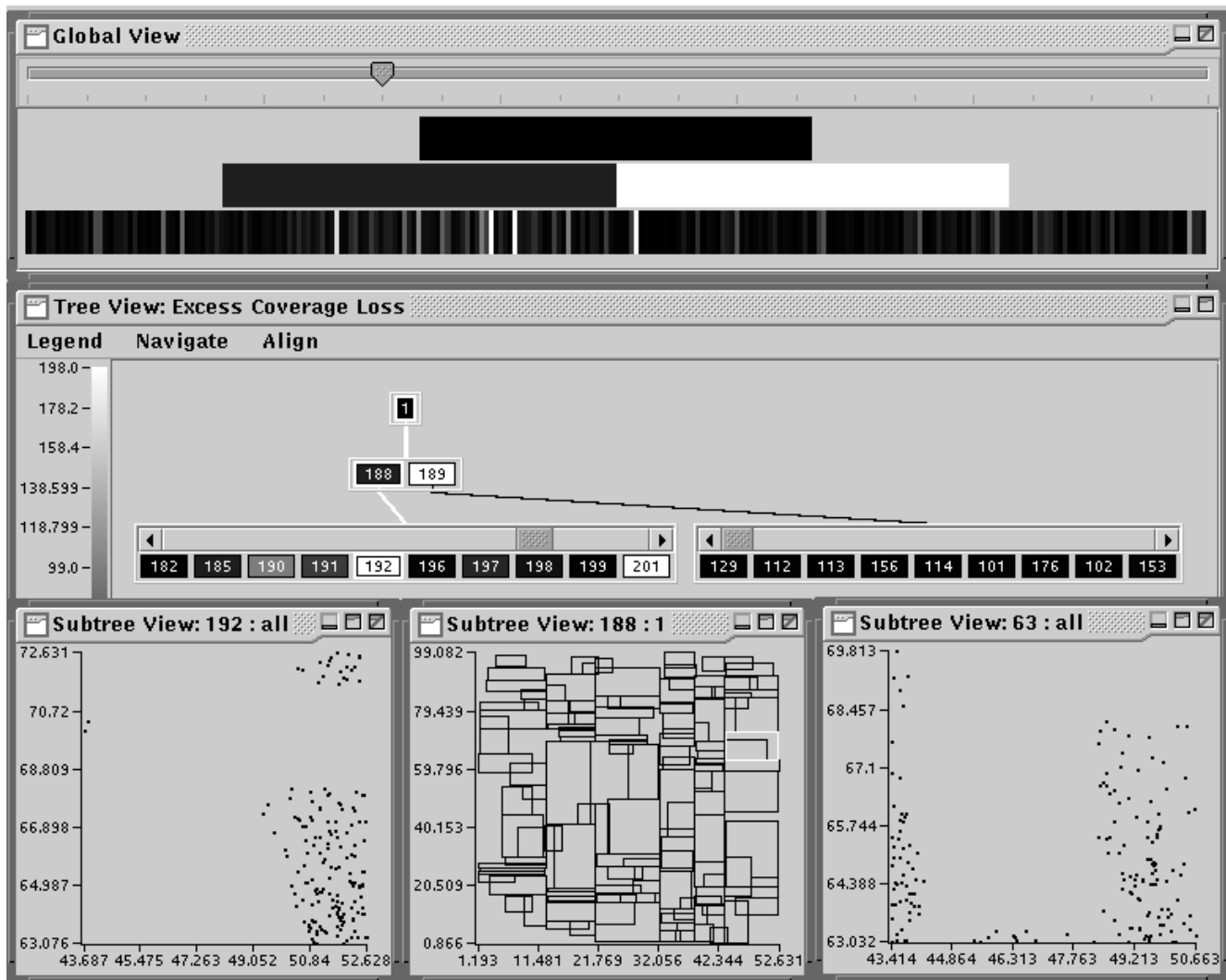
Figure 2. In this amdb session, we begin with the global view and narrow down upon the sources of excess coverage loss through the tree view to the subtree views. We discover the cause of high excess coverage loss for node 192 is high overlap with node 63. Thus, the SP or split algorithm are design aspects for further refinement.
