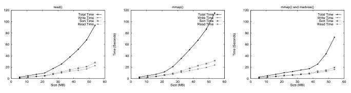
Figure 2: **Read() versus Mmap().** All three graphs show cumulative numbers for an UltraSPARC I with 64 MB of memory and one Seagate 5400 RPM disk. The first two graphs show that when read or mmap is used, the total sort time increases super-linearly before nearing the memory limits of the machine. The right-most graph shows that with memory mapping and advising, available memory can be used more effectively.
